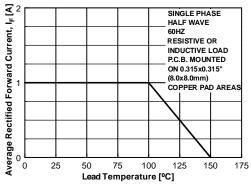
**Figure 1. Forward Current Derating Curve**
