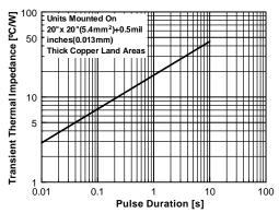
Figure 6. Thermal Impedance Characteristics
