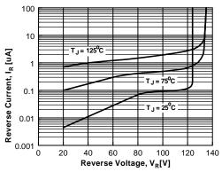
Figure 4. Reverse Current vs Reverse Voltage
