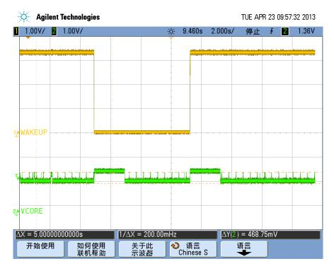
Figure 3-14 ats24=2, edge trigger, if no data after wake up, set to sleep mode again after 2s
