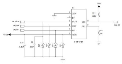
Figure 3-10 SIM card reference design
