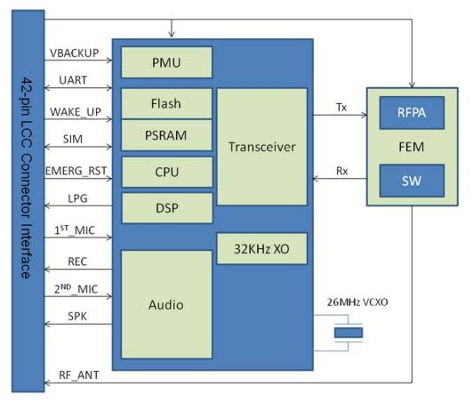
Figure 3-1 Block Diagram
