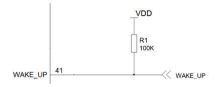
Figure 3-13 Recommended circuit for WAKE\_UP
