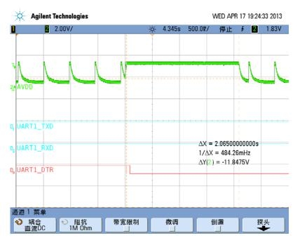
Figure 3-7 Pull down DTR, module wakes up 2s
