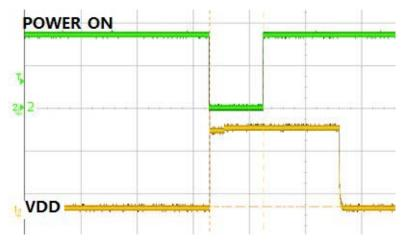
Figure 3-3 Failed to power on
