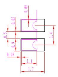
Figure 5-2 Recommended PCB layout
