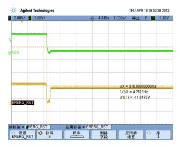
Figure 3-11 EMERG\_RST pull low, G510 reset peremptorily
