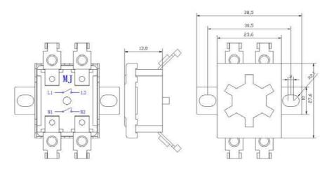
2.2 Terminal Strength: Terminals can bear tensile force of 80N and thrust of 800N.
