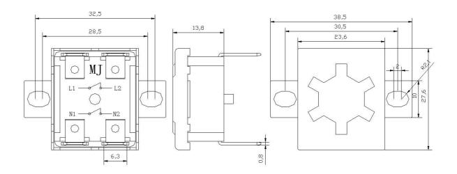
2.2 Terminal Strength: Terminals can bear tensile force of 80N and thrust of 70N.
