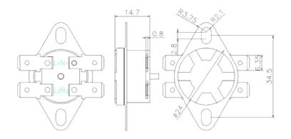
2.2 Terminal Strength: Terminals can bear tensile force of 80N and thrust of 70N.
