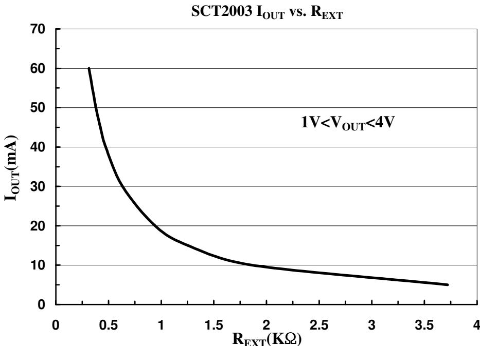
Furthermore, when SCT2003's output voltage is set between 1V and 4 V, the output current  $I_{OUT}$  can be estimated by the formula:  $I_{OUT} = 30(630 / R_{EXT})$  (mA) (Chip skew  $\pm 5\%$ ), Thus the output currents are set about 21mA at  $R_{EXT} = 900\Omega$ .
