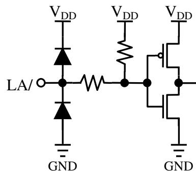
**Equivalent Circuits of Inputs (2)**
