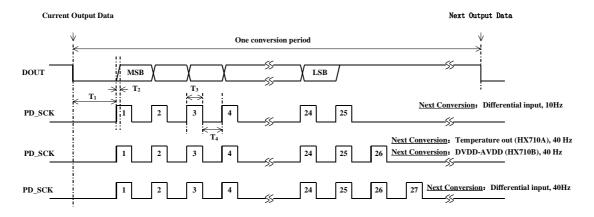
Fig.2 Data output, input and data rate selection timing and control
