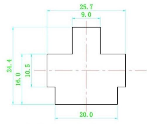
PANEL THICKNESS:1.0~1.5mm PANEL HOLE SIZE
