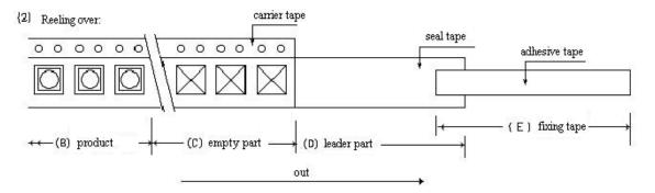
Last reeling empty part of carrier tape shall be more than 10cm.
