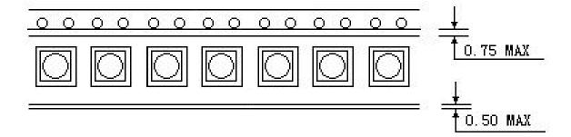
Deviation between carrier tape and seal tape shall be less than 0.5mm Seal tape shall not cover on the feeling hoes .
