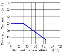
Fig.2 Forward Current Derating Curve
