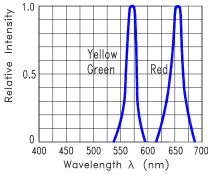
Fig.1 Relative Intensity VS. Wavelength
