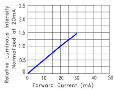
Fig.4 Relative Luminous Intensity vs. Forward Current
