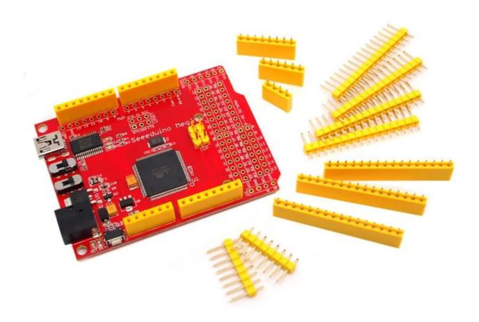
Built around ATmega 2560 @ 16MHz Massive GPIOs: 70 digital I/Os, 16 Analog input and 4 UART etc Small form factor, 30% smaller than Arduino Mega 3.3V and 5V dual mode Can be powered through a battery or through a AC to DC adaptor
