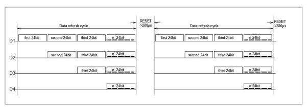
Note: D1 is the data from MCU, and D2, D3, D4 are from Cascade Circuits.
