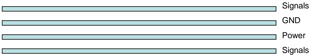
Figure 17: Typical 4-layer PCB construction
