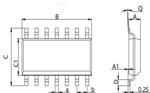
Dimensions In Millimeters (SOP14)
