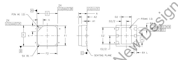
Figure 8. 3x3 6-pin DFN with Protective Cover
