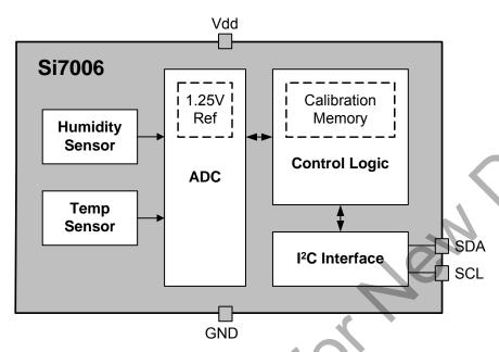
Figure 5. Si7006 Block Diagram
