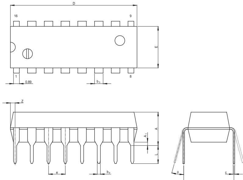
The technical drawings illustrate the physical dimensions of the DIP-16 package. The top view shows the overall width (D), height (w), and lead spacing (b<sub>3</sub>). The side view provides a detailed look at the lead profile, including lead thickness (e), lead pitch (e<sub>1</sub>), lead angle (θ), and lead height (c). A callout specifies '(Ni/Pd/Au plating)' for the lead surface treatment.
