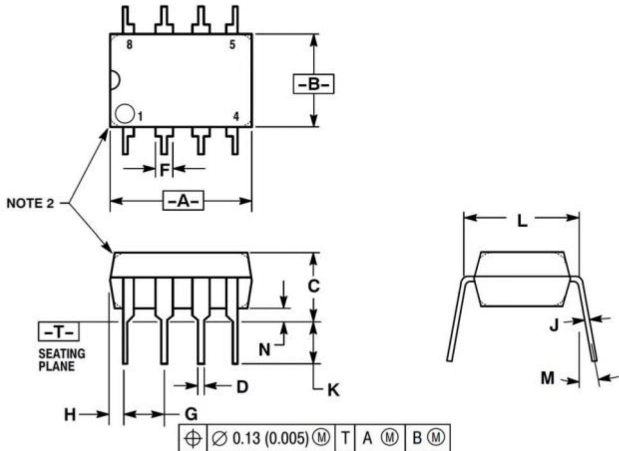
Note: 1. The L dimension is the dimension when the pins are parallel; 2. The shape has two rounded corners and square corners.
