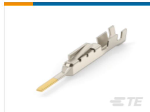
TE Part #1318111-1 Contact: Component To Wire ; 5A, 28- 18 wire size, gold plated
