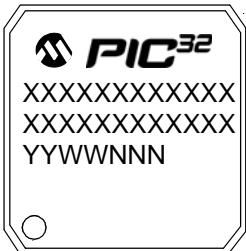
100-Lead TQFP (12x12x1 mm)
