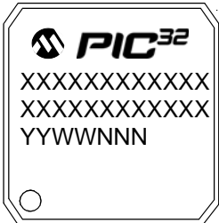
100-Lead TQFP (14x14x1 mm)
