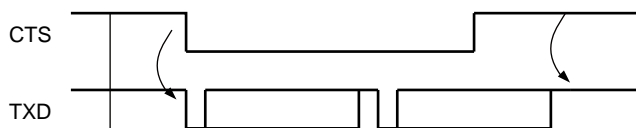
Figure 25-28. Transmitter Behavior when Operating with Hardware Handshaking
