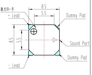
\*Unit: mm; Tolerance: ±0.3mm Except Specified
