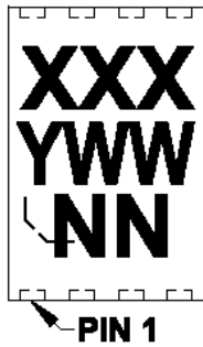
8-Lead TDFN (2x3x0.75 mm) ( MCP6V62 )
