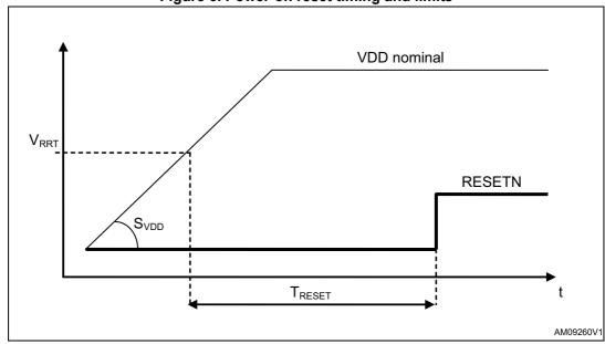
Figure 6. Power-on reset timing and limits
