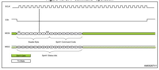
Concerning the first byte, the MSB is an A/C bit (Address/Commands: 0 indicates that the following byte is an address, 1 indicates that the following byte is a command code), while the LSB is a W/R bit (Write/Read: 1 indicates a read operation). All other bits must be zero.
