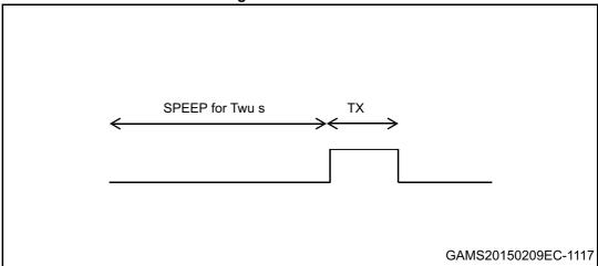
Since the embedded LDCR system automatically manages the transmission strobe, only a FIFO reload has to be done after the TX done IRQ (or in general, before the next wakeup) in order to prepare the next Tx.
