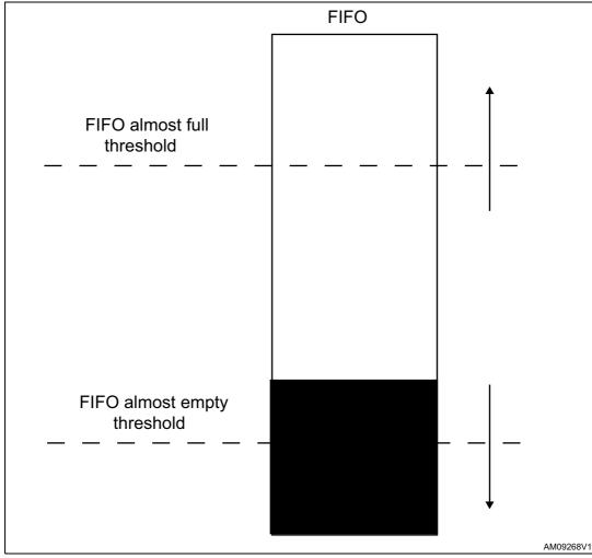
Figure 13. Threshold of the linear FIFO
