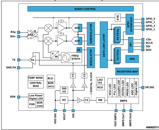
Figure 1. SPIRIT1 block diagram
