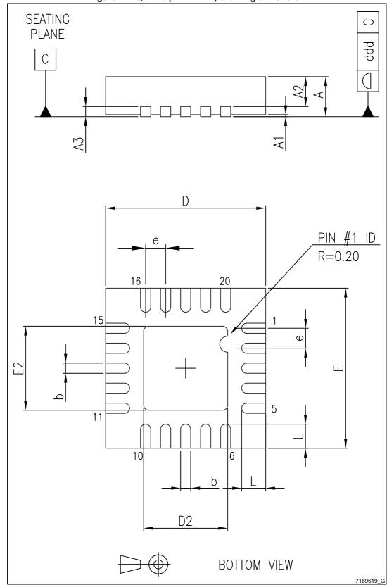
Figure 17. QFN20 (4 x 4 mm.) drawing dimension
