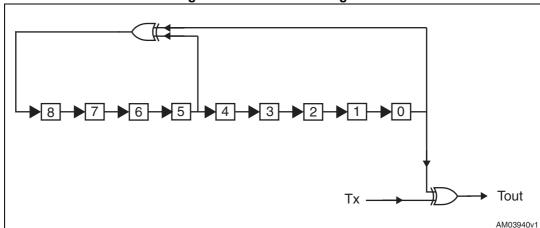
Figure 12. LFSR block diagram
