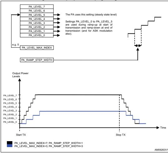
Figure 11. Output power ramping configuration
