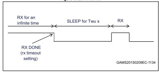
The wakeup timer for LDCR mode can be set through the LDC\_PRESCALER/COUNTER registers. This timer is clocked by the 34.7 kHz RC oscillator keeping unused blocks off.
