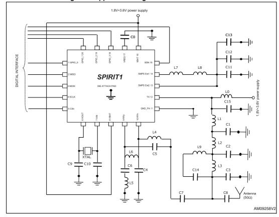
Figure 3. Application diagram for Tx boost mode
