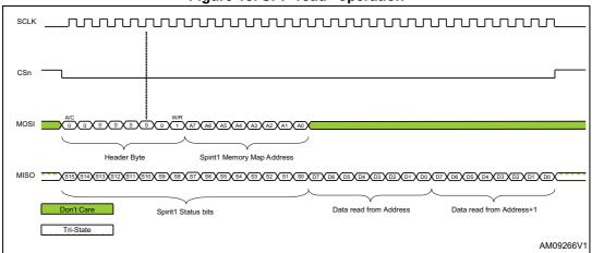
Figure 16. SPI "command" operation
