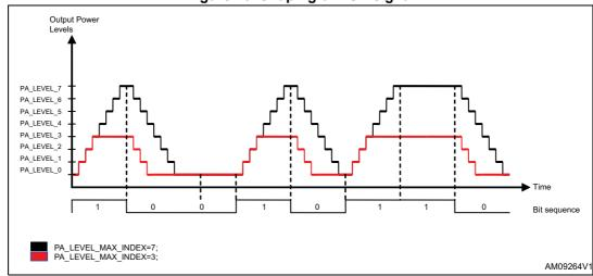
Figure 10. Shaping of ASK signal
