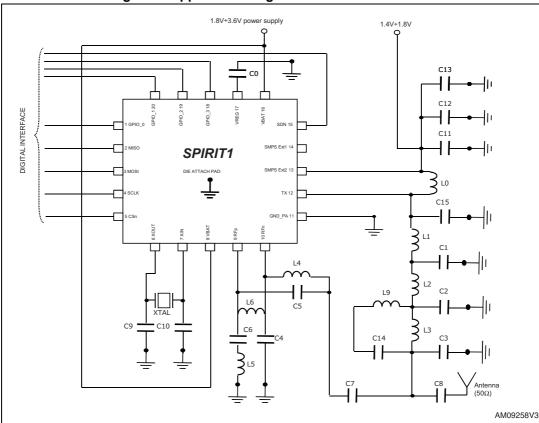
Figure 4. Application diagram for SMPS OFF mode
