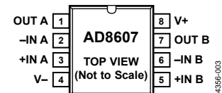
Figure 3. 8-Lead SOIC (R Suffix)
