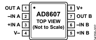
Figure 2. 8-Lead MSOP (RM Suffix)
